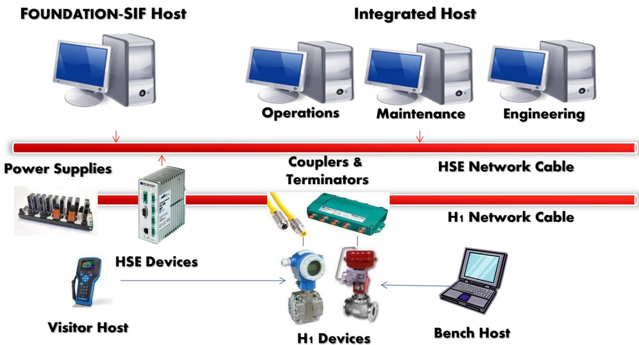
THE FIELDBUS FOUNDATION PROVIDES TESTING & REGISTRATION FOR ALL ELEMENTS OF A FIELDBUS SYSTEM FROM HOSTS TO CABLE TO DEVICES
