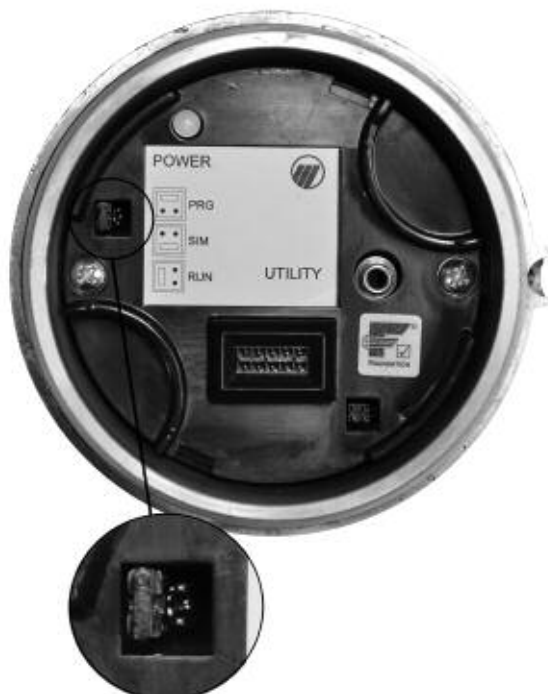
Remove jumper to disable simulation
